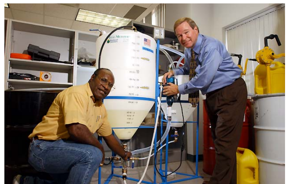
Figure 7. Transesterification of coconut oil into coconut bio-diesel
