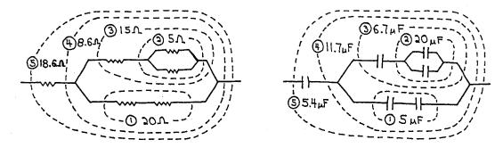
With circuits in "rectangular" format, it is difficult to see whether components are in series or parallel. Sometimes it helps to redraw a circuit in a visually logical "tournament bracket" style that is easier to analyze. Below, a circuit is re-drawn to make series & parallel relationships clear. { He circuits use the same re-drawing principles }
