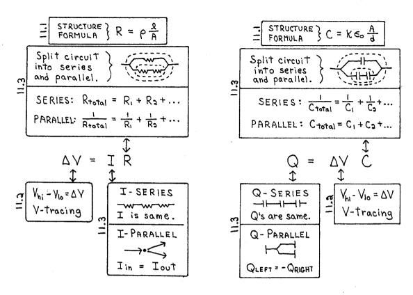
V=IR (or Q=VC) can be used for each individual  $\checkmark$  (or  $\dashv$ ), or for any combination.
