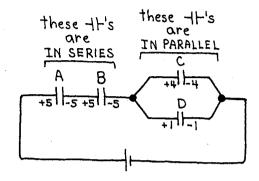
A capacitor's + and - plates always have equal-and-opposite charges. This is shown above: +5 & -5 are equal-and-opposite, so are +4 & -4, and +1 & -1.
