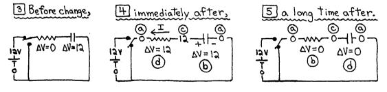
BEFORE THE SWITCH IS CHANGED, the situation is the same as in the "Charging" Picture #3. The  $\dashv$  is fully charged, with  $\Delta V = 12V$ .
