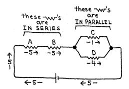
If resistors are in series, the same current (in this case, 5A) flows through each , like the steady flow of water through a pipe. (The analogy to familiar flowing water may help you clearly visualize the impossible-to-see, yet very real, flow of charge through a wire.)
