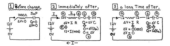
BEFORE THE BATTERY IS CONNECTED: Q = VC and Q = 0, so  $\Delta V$  across the  $\dashv \vdash$  is 0.
