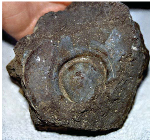
Figure 3. Photo of supposed iron washer with central mashed rivet but which, in reality, is a coating of cemented magnetite grains altered partly to limonite. 8 (Image published by Wyatt Archaeological Museum. 9 )
