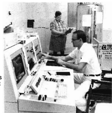
Ann Hunt stands near the magnet (11.7 Tesla) while fellow ASA member Richard Justice operates the computer of a 500 MHz NMR spectrometer at the Lilly Research Laboratories.
