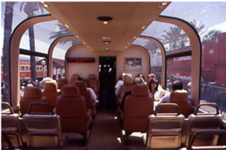
SMART-type self propelled vehicle with wrap-around glass
