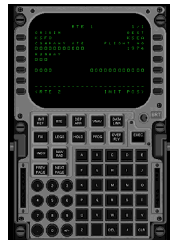
FMS Control-Display Unit
