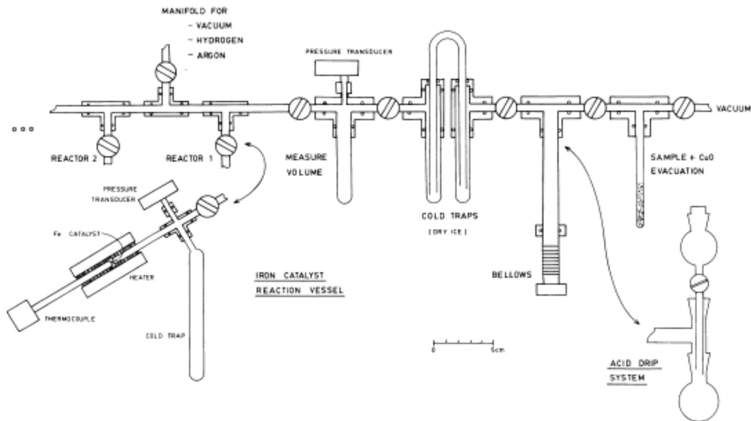
Fig 1. Multiple reactor apparatus for the graphitization of CO<sub>2</sub> over an iron powder catalyst. The volume of the reaction vessels could be varied by using different sized cold traps. Reaction volumes as small as 3ml were possible.
