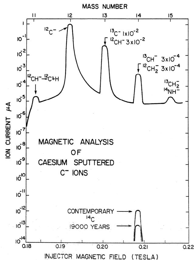
Fig 16.2. Magnetic analysis of the negative ions sputtered from a carbon target
