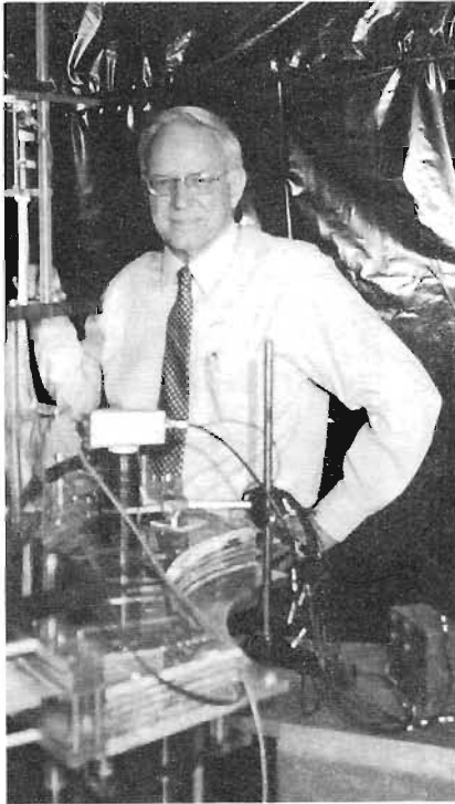
Jack McIntyre in his Texas A&M University laboratory, running tests on his "PET Project." Foreground: Quarter ring of the scanner designed and constructed in the lab. (Read his lips: "This thing is going to work!")
