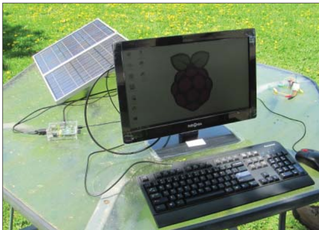
An experimental setup for a solar-powered Raspberry Pi.
